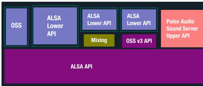
Figure 4-3. ALSA and PulseAudio. This diagram is upside down compared to mine
